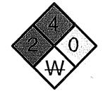
**Step 2:** Obtain current edition copy of NFPA 704 or view on line at www.nfpa.org/704. Compare the criteria on the SDS sections as shown above with the criteria shown in Tables 5.2 (Health), 6.2 (Flammability), 7.2 (Instability) and 8.2 (Special Hazards).
